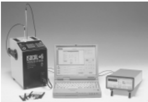
Fig 37: General Purpose Calibration System using a dry block calibrator
